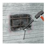
Step 3: Application of corrosion Protection layer Sika® Rustop/ SikaTop®-Armatec-108/ SikaTop®-Armatec-110 EpoCem®
