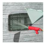
**Step 4:** Application of Concrete protection Solution **Sikagard® XT/ Sikagard® 550 W Elastic/ Sikagard® PU UR**
