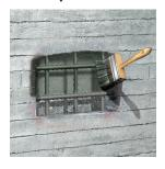
Step 5: Application of Repair Mortar Sika MonoTop® 122 F/ SikaTop®-122 HS/ SikaRep® Microcrete-3 UW/ SikaRep® Microcrete-4/ Sikadur® 41
