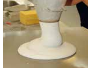
At compressive strengths above 150 MPa one is no longer concerned with commonplace concrete. Stone aggregates are replaced for example by fine aggregates of ceramic origin, and the entire binder matrix is only slightly reminiscent of classical concrete. Shown in the illustration is the flow behavior of a UHPC of 200 MPa.
