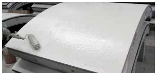
Immediately following curing in a steam channel, the concrete surface of tunnel lining segments is coated with water-based epoxy emulsion that is absorbed even into the smallest pores, thereby generating a sealed, protective coating.
