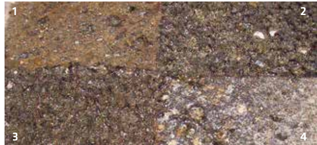
Fire exposure trials for concrete containing various aggregates. Surface spalling and sintering, and a range of temperature developments at differing depths can thereby be compared.
