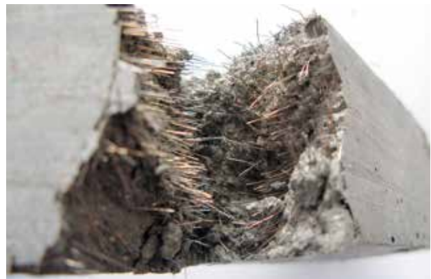
High strength and above all ultra high strength concrete are practically always also fiber-reinforced. Depending on the requirements, synthetic and/or steel fibers are thereby employed in large quantity. The high flexural strength of UHPC can be achieved in this way.
