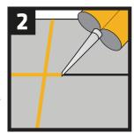
3. As soon as possible after application, smooth the grout with a finishing tool (metallic ball) to obtain a smooth finish.
