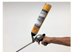
6. Apply SikaRoof<sup>®</sup> Board Adhesive directly onto the surface, then quickly press the insulation panel onto the flat roof with light pressure and adjust. Use the spacer to ensure right distance between the nozzle and a substrate.
