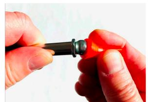
SikaRoof<sup>®</sup> Board Adhesive is ready to use. The amount of expanding foam can be adjusted by applying more or less pressure on the trigger.
